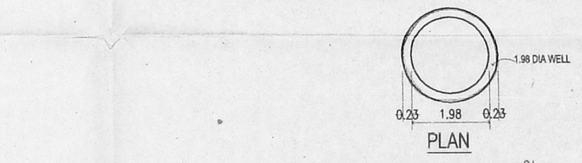
SECTION DETAIL OF FOUNDATION
